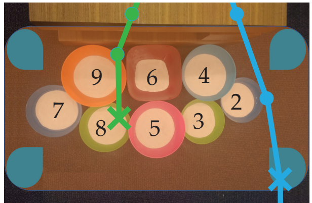
Fig. 6. Top view of the eight targets in the variant of mini-golf user study. The users assign distinct scores from 2 to 9 to the targets. The figure shows an example of this ranking. While the robot is capable of hitting the ball into the entire shaded region, the maximizers of a linear reward always lie near the corners of the shaded region in blue. Therefore, while the GP reward model can query the user with better trajectories (e.g. the green trajectory), the linear model only explores the boundaries (e.g. the blue trajectory that throws the ball outside of this region). Crosses show where the ball hits the ground.
