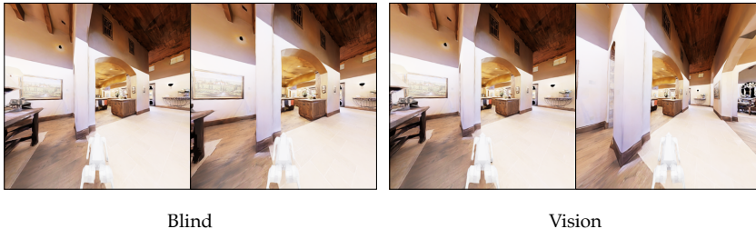
Figure 9: Comparison between Go2 blind policy and vision policy. The blind policy failed to avoid the obstacles and got stuck. The vision policy detected the obstacle and got around to avoiding it.
