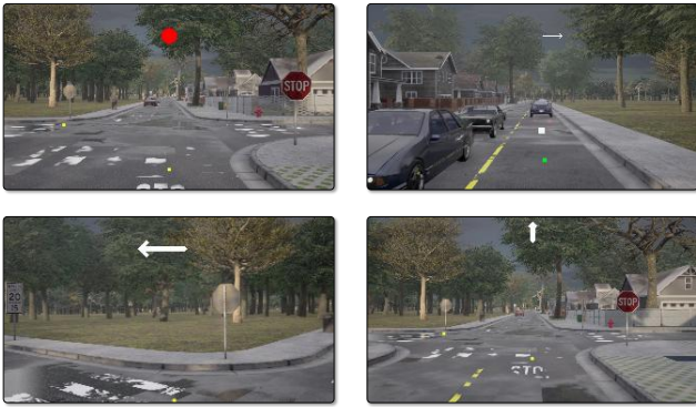
Fig. 3: Confounded overlay visualization in the CARLA simulator. Action-conditioned icons are rendered along the top margin of each frame to induce spurious correlations, while leaving the underlying dynamics and expert labels unchanged. The red circle simulates a brake light, while arrows denote the steering direction, with their thickness indicating the throttle applied in the previous timestep.
