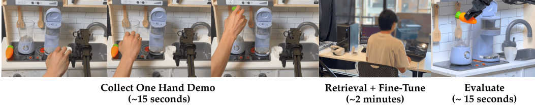
Figure 11: Fast Adaptation. We conduct a small-scale user study to demonstrate HAND 's ability to learn robot policies in real-time. From providing the hand demonstration (Left), to retrieval and fine-tuning a base policy (Middle), to evaluating the policy (Right), we show that HAND can learn to solve the Put Carrot in Blender task with 7.5/10 task completion in less than 3 minutes.
