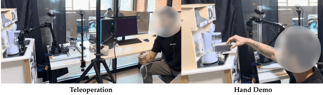
Figure 10: Efficient Demonstrations. Two users, unfamiliar with HAND are asked to collect trajectories either via teleoperation (Left) or using their hands (Right). HAND retrieval achieves a 50% success rate with the same amount of demonstrations using 3\times less time. STRAP retrieval is unable to reach 50% even when provided with more expert demonstrations.
