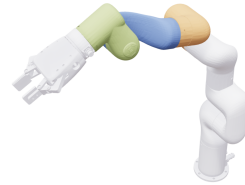
Figure 3: Contact links. Collision meshes of the xArm 7 forearm (link 4), wrist yaw (link 5), and wrist pitch (link 6) form the contact surface \mathcal{M} .
