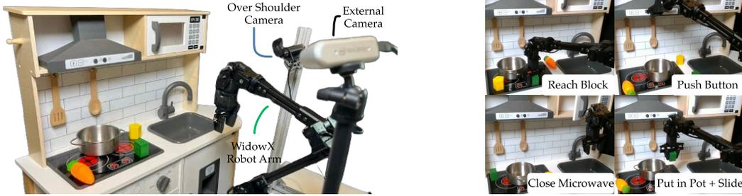
Figure 2: **WidowX Robot Arm Setup and Evaluation Tasks.** We evaluate the scalability of CLAM using four manipulation tasks (Right) on a WidowX robot arm (Left) in a toy kitchen setup [24].
