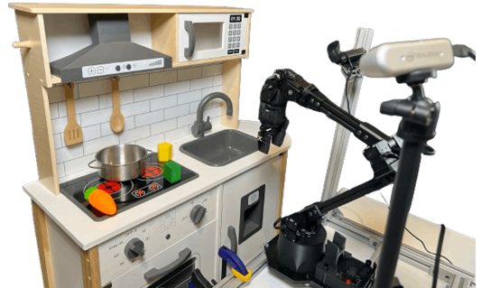
Figure 4.3: WidowX Robot Arm Setup. We evaluate the scalability of HAND on 10 manipulation tasks on a WidowX robot arm in a kitchen setup [292].
