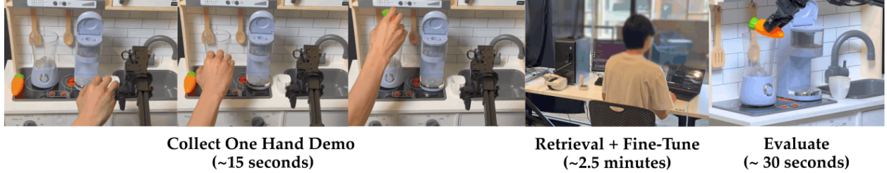
Figure 4.5: Fast Adaptation Study. We conduct a small-scale user study to demonstrate HAND’s ability to learn robot policies in real-time. From providing the hand demonstration (Left), to retrieval and fine-tuning a base policy (Middle), to evaluating the policy (Right), we show HAND can learn to put a carrot in the blender with 7.5/10 task completion in less than 4 minutes.
