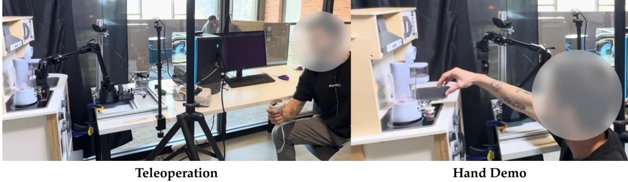
Figure B.5: Efficient Demonstrations. Two users, unfamiliar with HAND are asked to collect trajectories either via teleoperation (Left) or using their hands (Right). HAND retrieval achieves a 50% success rate with the same amount of demonstrations using 3× less time. STRAP retrieval is unable to reach 50% even when provided with more expert demonstrations.
