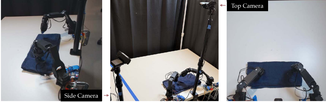
Figure 11: Real World Bimanual Robot Setup. Our real-world setup consists of a top-down and side camera mounted to a table where two Koch v1.1 low-cost arms are mounted. This setup allows us to perform bimanual tasks and easily collect data with another pair of low-cost “leader” arms mounted to the same table.
